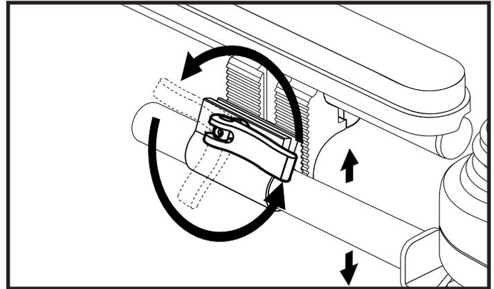
Figure 20. Controller Height Adjustment (Two Post and Heavy Duty Drop-in Armrests)
