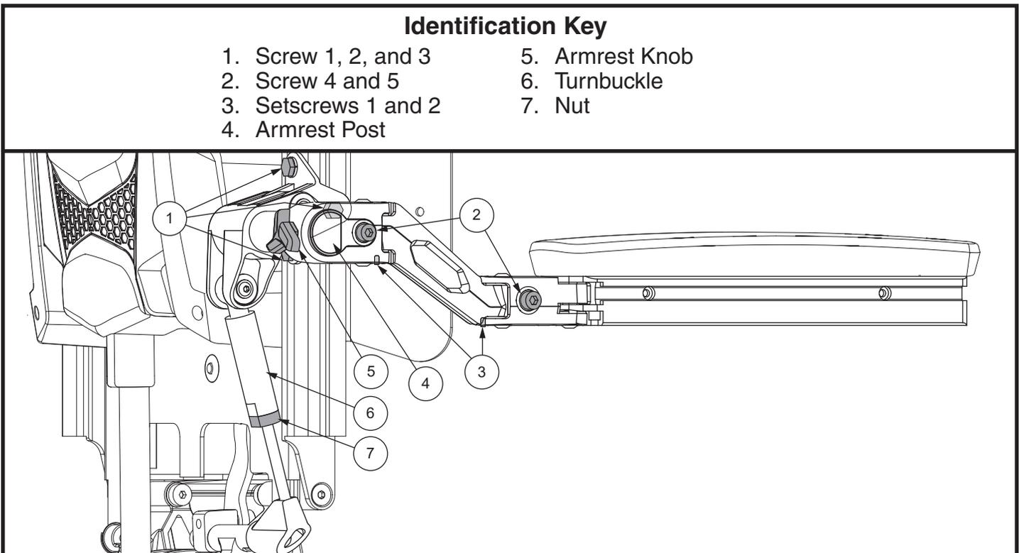
**Figure 9. Flip-up Armrest Height and Angle Adjustment**
