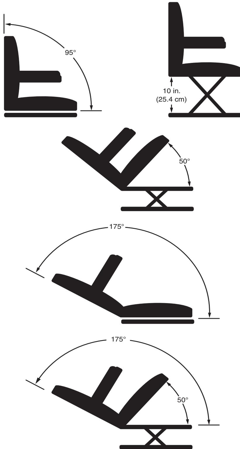
Figure 3. TRU-Balance® 3 Power Positioning System Range of Motion
