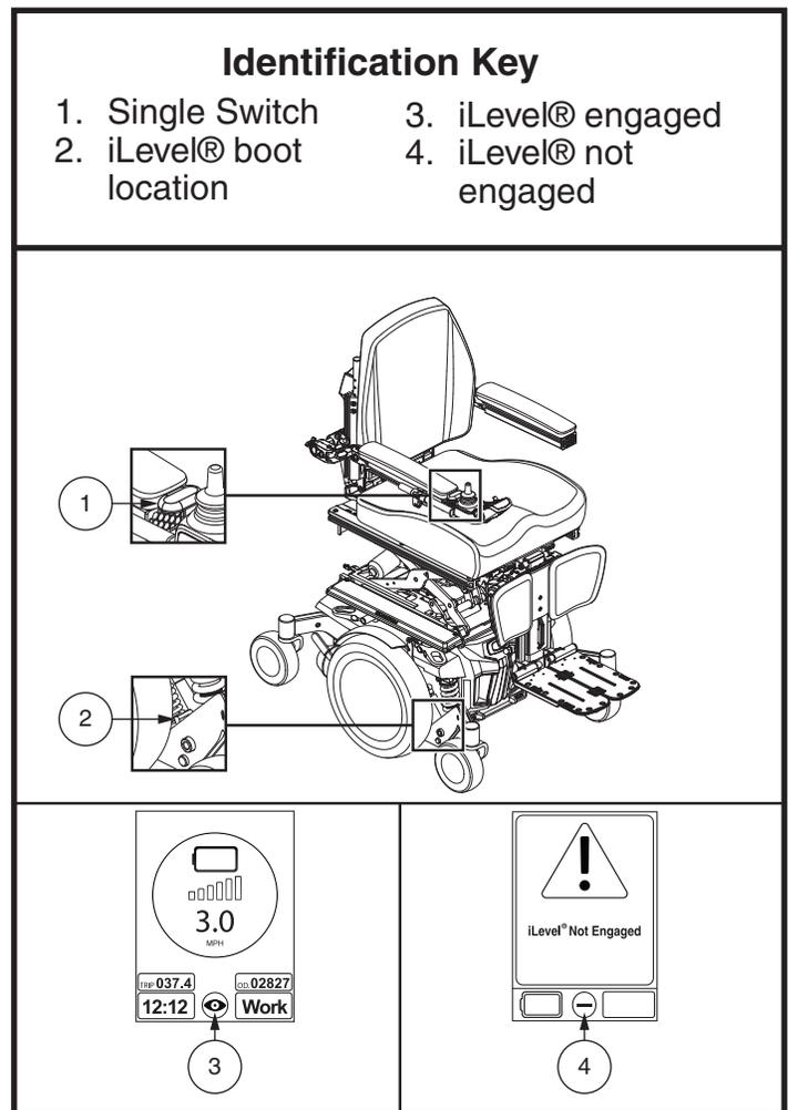
**Figure 4. TRU-Balance® 3 with iLevel® Feature and Controller Indicators**
