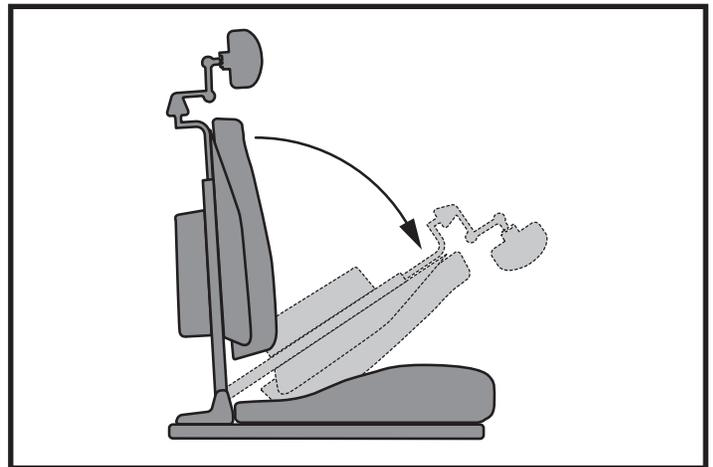
Figure 5. Flip-forward Back (Disengaged)
