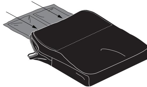
**Figure 5. Essence Plus ASPP Polyurethane Liner—Top of Cushion**
